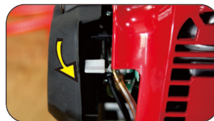
9. Turning on choke lever.
