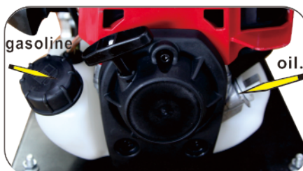
5. Firstly pouring in the gasoline, then pouring in the engine oil.
