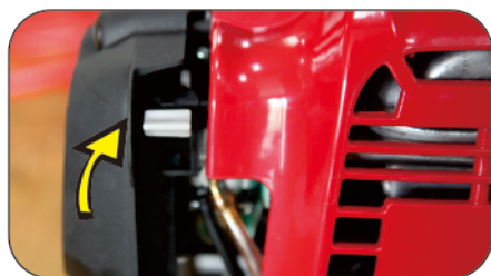
7. Turning off the choke lever.
