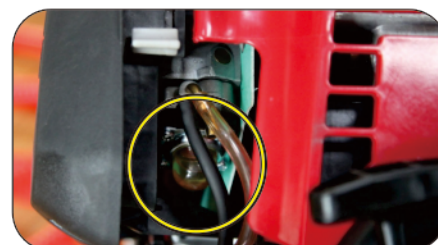
6. Pressing the oil bubble to fill up with gasoline.
