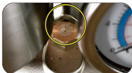
4. Tearing off the sealing sticker.
