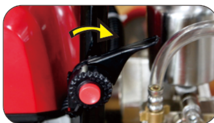
11. Increasing the throttle lever to suck the water (the right outlet will exhaust the air to fill up with the water on pump).
